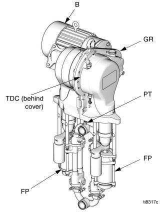
FIG. 1. E-Flo Electric Circulation Pump
